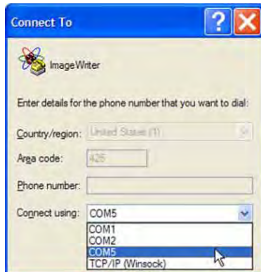
Figure 2-19— ImageWriter Will Usually Be the Highest Number COM Port If You Just Plugged It into Your Computer
