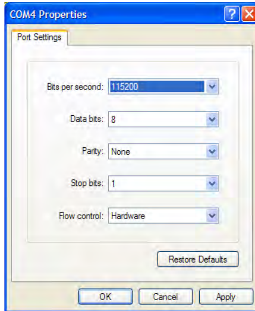
Figure 2-20—Factory default communications settings for IW are 115200, 8, N, 1 . FLOW CONTROL should read Hardware .
