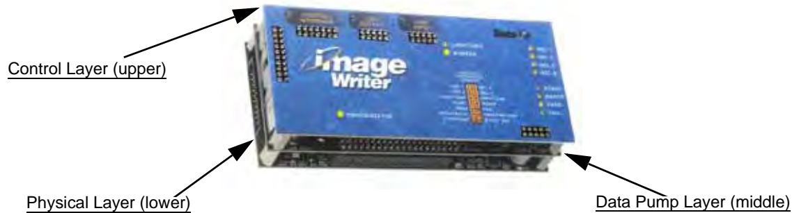
Figure 1-5—IW-300 Showing Three Layers of Hardware
