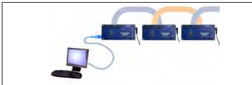
Figure 2-13—Link Networked ImageWriter-300s : One Master IW-300 and up to 31 Linked IW-300s
